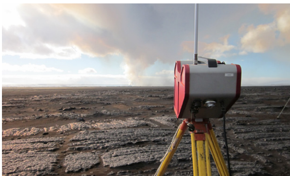
(Left) Infrared imaging camera (nicAIR-II) measuring close to the active lava from at Holuhraun. The camera was able to measure SO 2 gas at relatively high frequency (~ 1 Hz) and estimate mass loadings and emission rates. (Right) Example of an SO 2 retrieval from the Holuhraun gas plume. Mass loadings were extremely high (>5000 ppm*m) and in some places saturation occurred.
