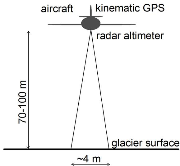
Figure 2. Upper: Surveying aircraft of Isavia with installations of surveying equipment for monitoring, including the radar altimeter used for surface profiling (from Gudmundsson et al. 2015, Deliverable 7.2). Lower: geometry of altimeter beam spreading at optimal flying height of 70-100 m (after Gudmundsson et al. 2007).
