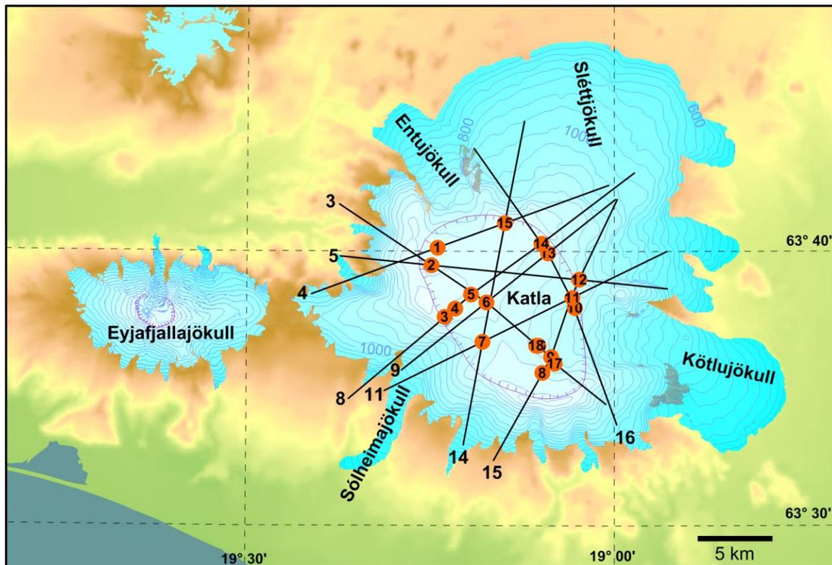
Figure 10. Survey lines accross Katla, used for aircraft altimeter surveys 1999-2015.
