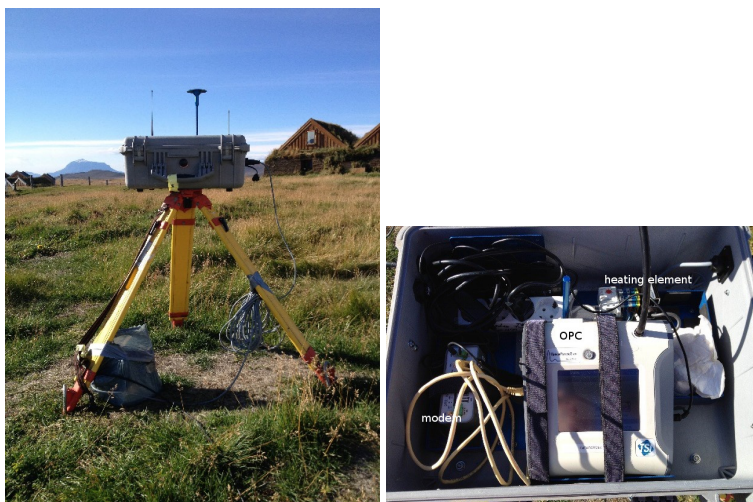
Figure 8: a) The OPC is measuring in Möðrudalur in September 2014, and b) Look inside of the enclosure.
