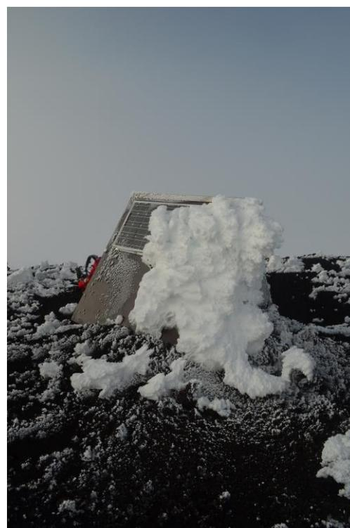
Figure 3: Icing after 3 days in spring conditions
