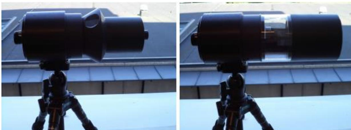
Figure 10: The standard conical scanner with a rotating hood and a small quartz window can be seen to the left and the prototype scanner with a non-rotating quartz window can be seen to the right.
