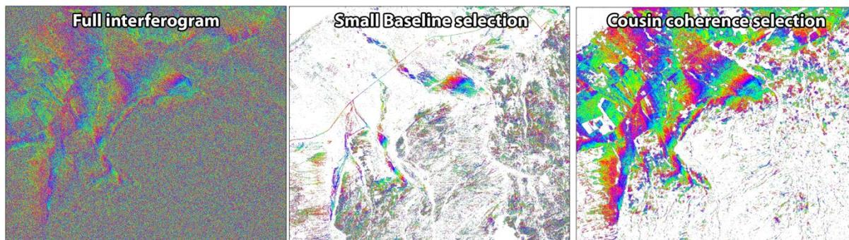
Figure 1.6: Demonstration of point selection in an interferogram affected by snow (20100204-20100331): Full interferogram (left), point selection using Small Baseline method (middle) and cousin coherence selection (right).
