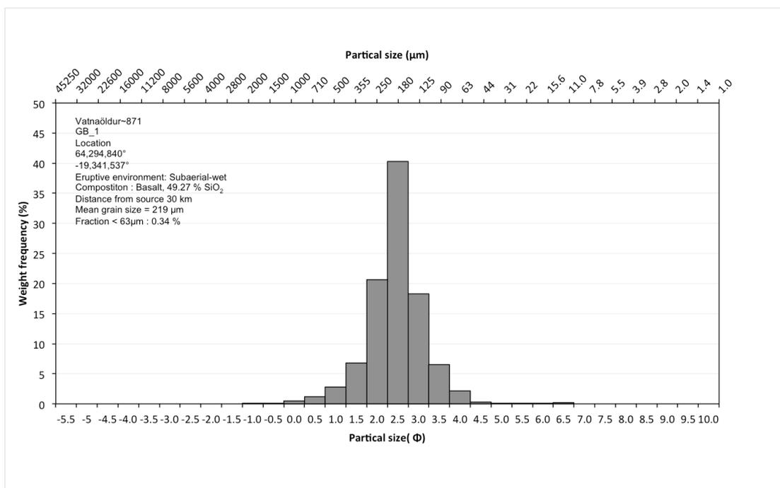
Figure 2: Example of a figure showing grain size distribution for the 870 CE eruption of Bardarbunga. Newly analysed grain size data are included in the database in order to describe a full range of likely eruption scenarios in Iceland.
